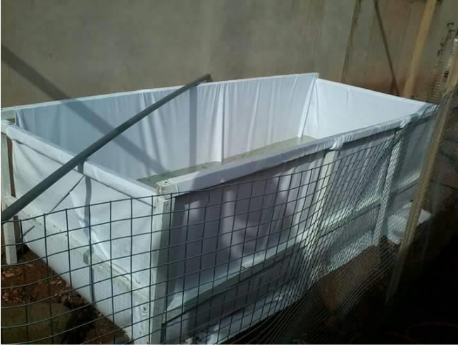
Picture 3: Tarpaulin Tank (Locally fabricated with wooden frame)
