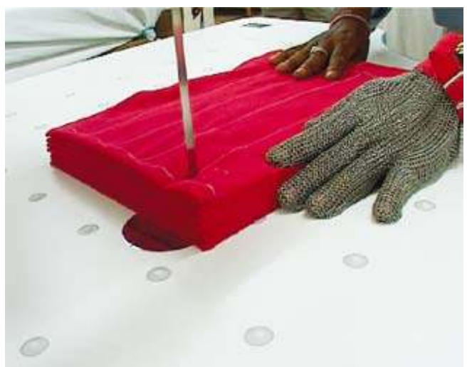
Then the whole bunch of cloth is cut together with this kind of 'sawing' machine
