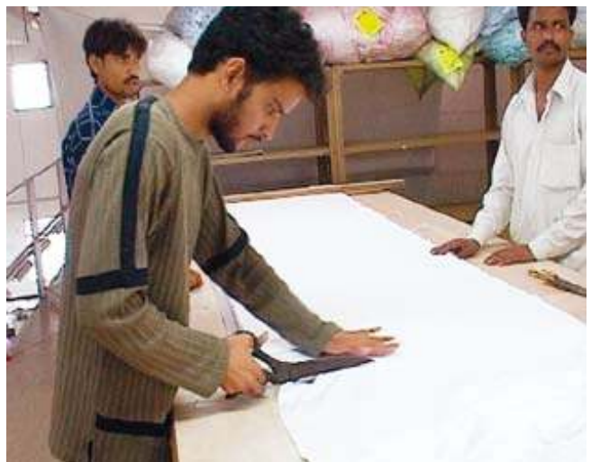
Clothes being prepared for cutting. 20 to 50 pieces are joined together.
