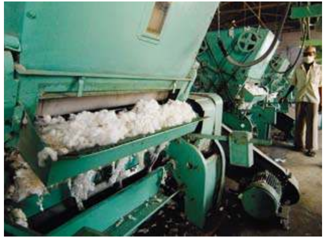
The cotton quality is assessed by bioRe's procurement officer, the same person who goes from house to house. Cotton seeds – the name used before ginning – will lose two-thirds of its weight through extracting the seeds. The remaining fibres are called cotton lint.
