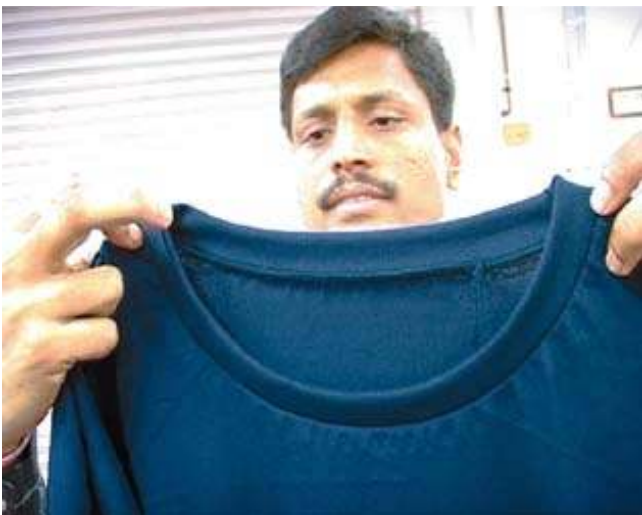
For making a neck, two very different parts are stitched together
