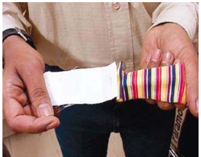
A textile should not shrink nor de-colour. The sample (right) is tested with a fabric in a washing machine.
