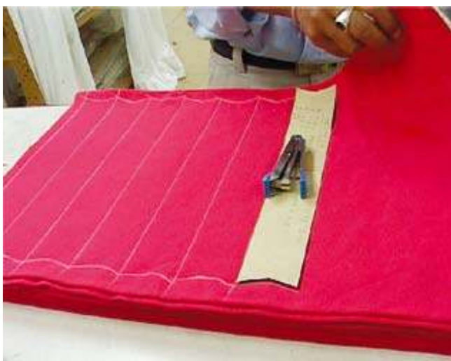
Depending on the cutting pattern, the different parts are marked with a white pen on the top cloth
