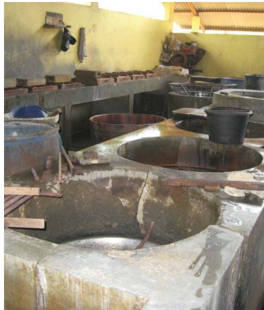
New stainless steel vats (left) and traditional set-up (right).
