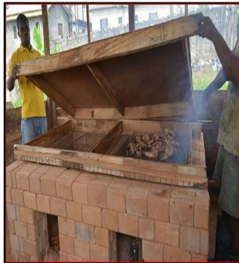
Chorkor Oven for fish drying
